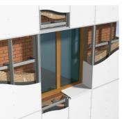
A ventilated facade is a structure that provides ventilation of the space between the exterior cladding and insulation.
